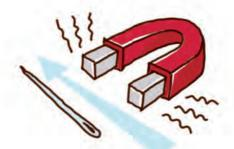
1 Move the magnet over the needle about 10 times. Always move it in the same direction. This way the needle becomes a magnet, too.
